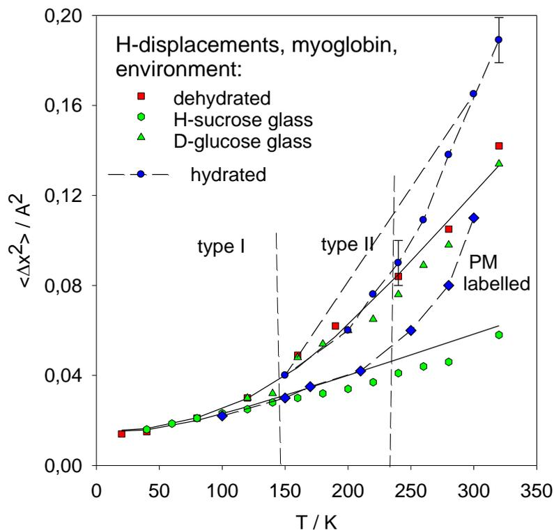
*Fig. 1: mean square displacements (IN13,  $\tau_{res} = 140$  ps) of myoglobin in various environments: dehydrated (red squares), hydrated (blue circles), green triangles: per-deuterated glucose glass, green circles: D/H-sucrose glass<sup>10,2</sup>, blue diamonds: H-labelled per-deuterated PM fragments<sup>10</sup>, line: calculated vibrational displacements<sup>16</sup>. The onset temperatures at 150 K (I) and 240 K (II) are indicated. (PM = purple membrane)*
